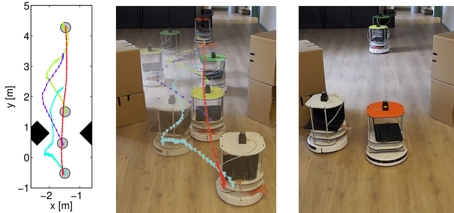
Figure 6.19: COCALU_{CP} with three turtlebots and an uncontrolled moving obstacle. The three controlled robots are located together on one side and the uncontrolled robot is on the other side. Some robots still have to pass through the small passage defined by the two static obstacles. On the left the left a trajectory plot is shown of the following the poses reported by the robots' AMCL, since no external ground truth localization method is available. In the middle, the same trajectories are overlaid on a picture of the actual run. The right most picture shows the situation that the white robot waited until the red uncontrolled robot passed so that it is free to move to the passage.
